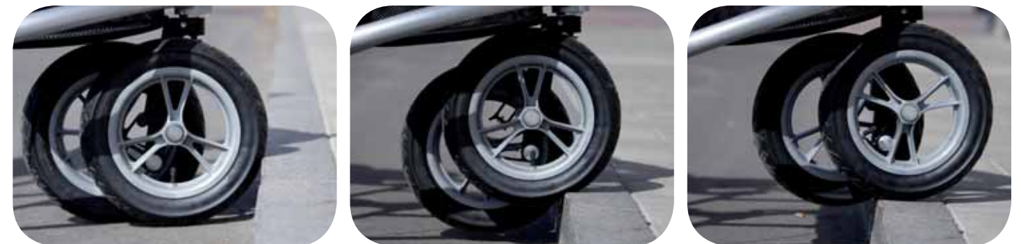
The Trionic Climbing Wheel in action overcoming a 13 cm high curb.
